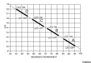
Fig. 77 - Outside Air Temperature Changeover Setpoints
